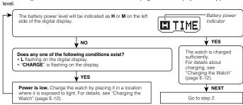
When L is flashing, the second hand will jump at two-second intervals.
